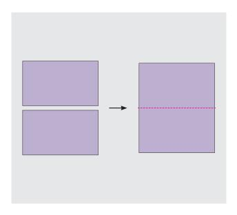
The back can also consist of 2 stripes W  $165 \times H 100 \times C$  cm each. The frame on the back is omitted.
